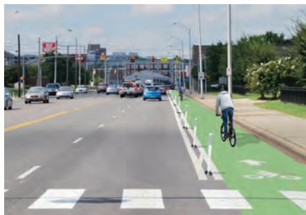
Above: Conceptual illustration of Charlotte Avenue with dedicated bike rapid transit infrastructure, including buffered lanes and flexible bollards for increased protection.
